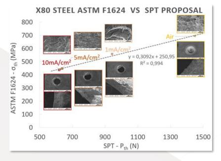
Pth, from tensile specimens is converted into oth and plotted into a graph **oth vs Pth-SPT**
