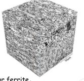
Ferritic microstructure with grain size range 5-15 $\mu$ m with some degenerated bainite/pearlite and no acicular ferrite.
