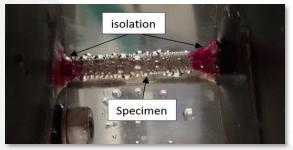
The specimen areas coincident with the wall passages were coated with an insulating varnish.
