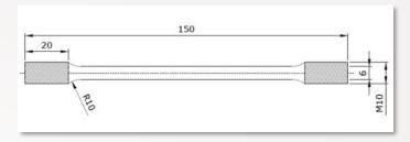
A set of  $\emptyset$ 6mm cylindrical specimens were obtained from an X80 plate in TL orientation
